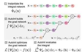
Figure 2. AutoInt pipeline. After (1) defining an integral network architecture, (2) AutoInt builds the corresponding grad network, which is (3) optimized to represent a function. (4) Definite integrals can then be computed by evaluating the integral network, which shares parameters with its grad network.
